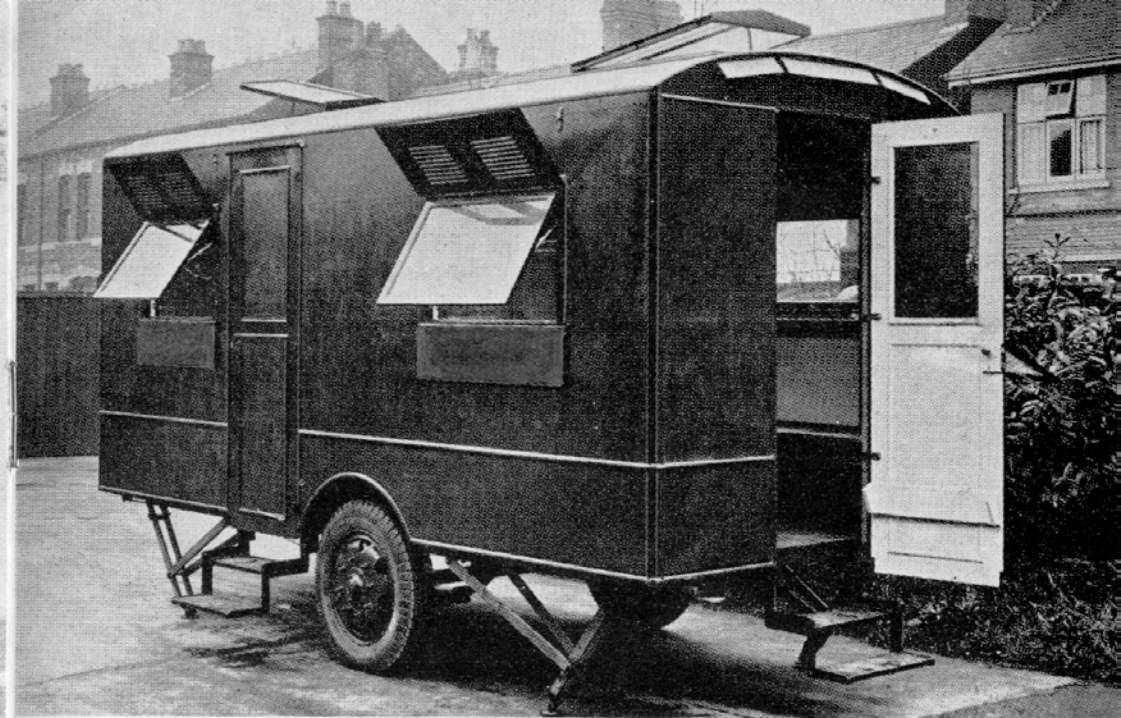
Shown above is a special purpose caravan submitted to the War Office in 1937. This was designed to provide working and sleeping accommodation for Staff Officers in the field. An order was eventually placed for caravans of this type
