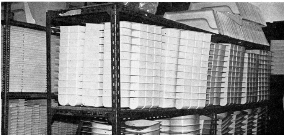
Eccles make their own vacuum formed plastic components for caravans.
