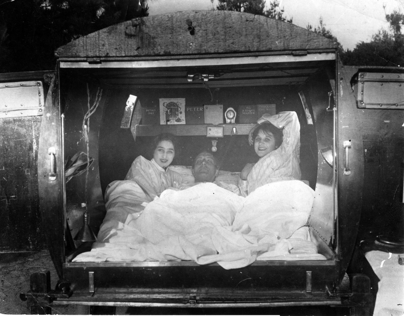
1916 Automobile Telescope Touring Apartment by de Bretteville, San Francisco. This is on a car chassis; on site storage boxes slide out of the main body like a chest of drawers, revealing a monster bed occupying the interior.
