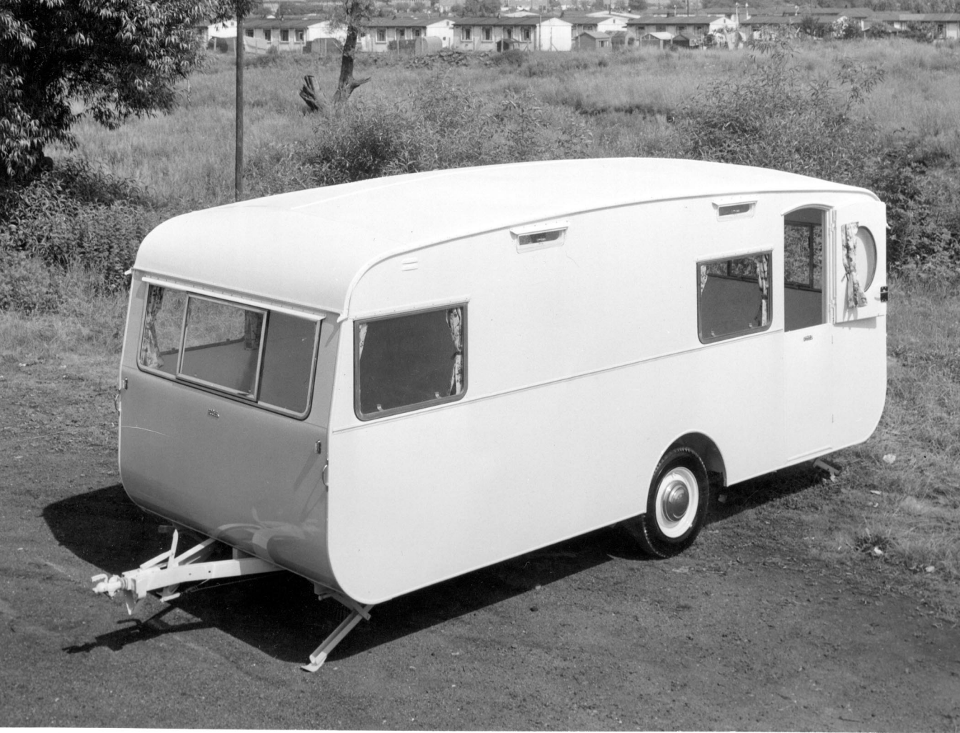
1959 Eccles "Leader" 17ft 6in, 4 berth, 1 double, 2 singles, end kitchen and toilet. Weight 19.5cwt. Price £430 ex wks
