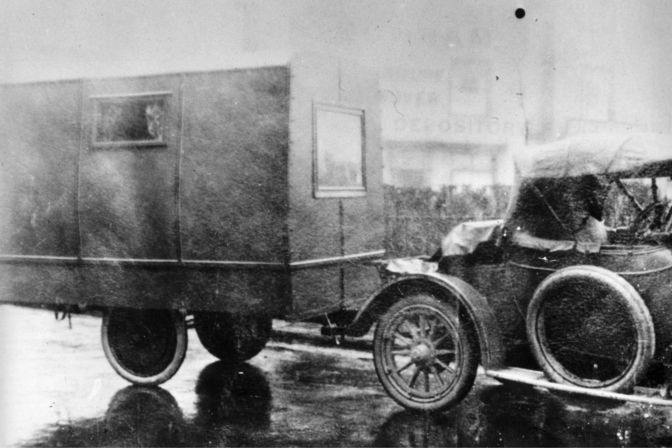
HCC Note - Picture captioned "1919 first Eccles Trailer, steel body" However it is different to model widely publicised as first trailer Side skirts over wheel where other steps in. Wheels are disc not artillery, front panel seams different.
